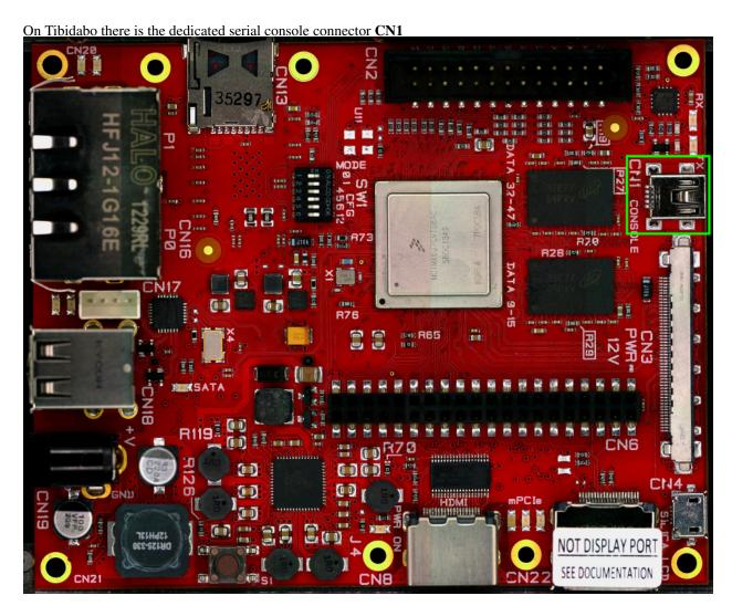
which you can connect, by means of a mini-USB cable, to your personal computer.
